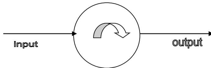
The isolator, shown in Fig. can be derived from a three-port circulator by simply placing a matched load (reflection less termination) on one port.
