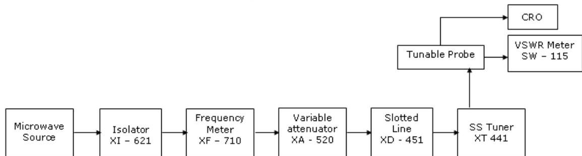
**FIG: SET UP FOR HIGH VSWR MEASUREMENT**
