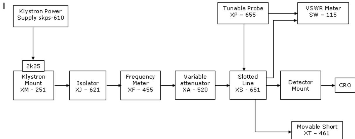
**FIG: SET UP FOR FREQUENCY AND WAVELENGTH MEASUREMENT**
