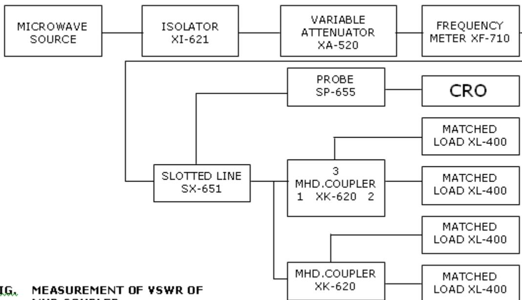
**FIG. MEASUREMENT OF VSWR OF MHD.COUPLER**
