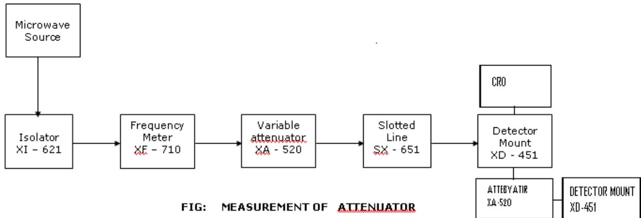
FIG: MEASUREMENT OF ATTENUATOR
